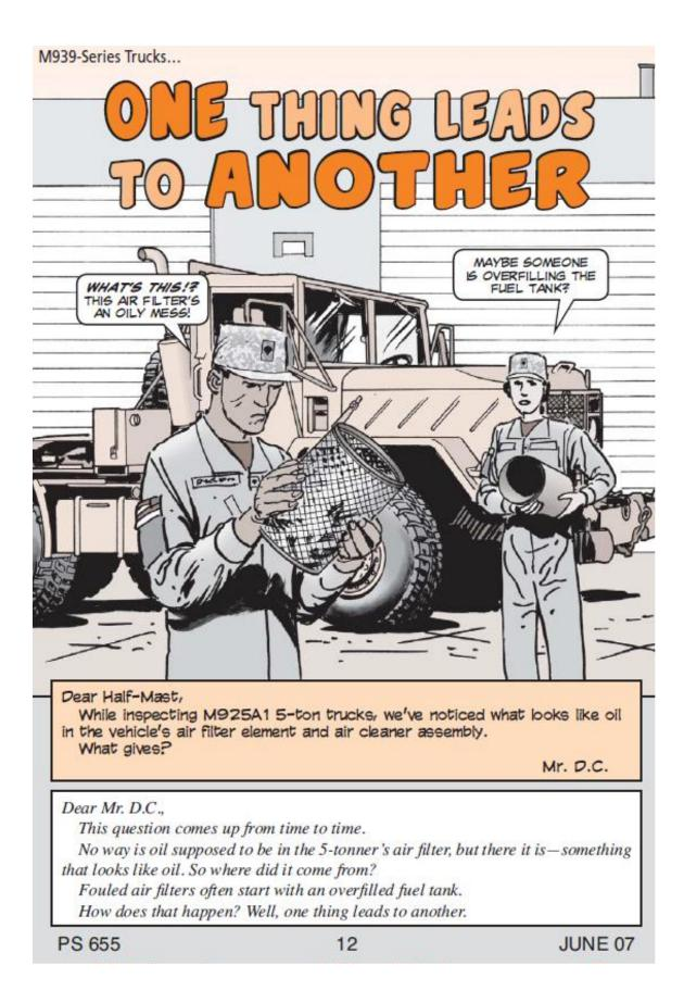
The fuel tank, transmission gear case and transfer gear case all vent into the air cleaner duct. Fuel from an overfilled tank can run through the vents and end up in the gear cases. Then, the fuel-oil mess from the overfilled gear cases is forced out through the vent lines... and ends up in the air filter.
